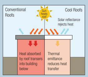
Solar reflectance and thermal emittance
