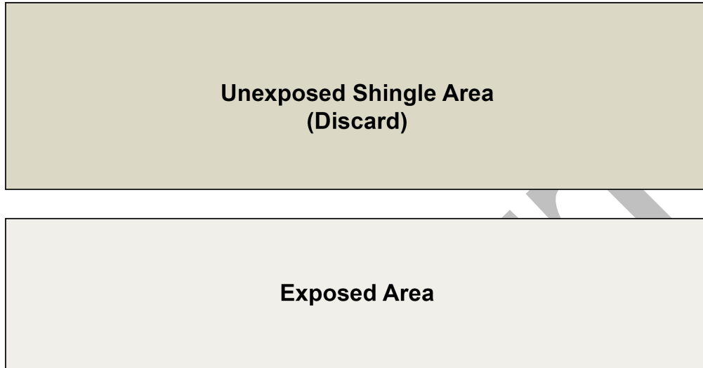
Figure 2. -Unexposed and Exposed Areas of Separated Shingle Board
