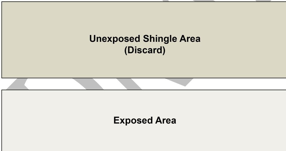
Figure 3. Unexposed and Exposed Areas of Separated Shingle Board
