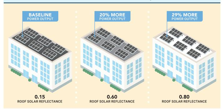
Examples of possible increases in bifacial PV power output as a result of raising a roof's SR. The SR values included in these examples are representative of low-slope roofing material options that were rated by the CRRC at the time of publication.
