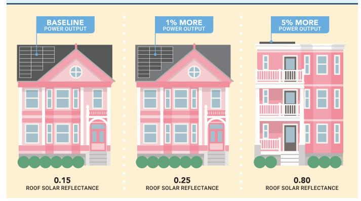
Examples of possible increases in monofacial PV power output as a result of raising a roof's SR. The SR values included in these examples are representative of steep- and low-slope roofing material options that were rated by the CRRC at the time of publication.
