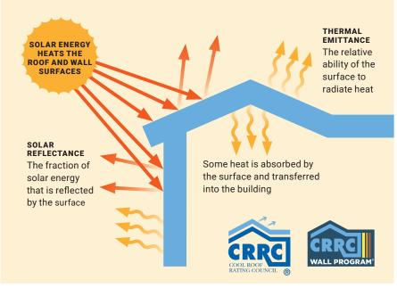
This illustration describes the flow of radiant energy as heat between the sun, roof and wall surfaces, building interior, and surroundings. The higher the solar reflectance, the more solar energy is reflected away from the surface. Some of the solar energy is absorbed by the surface as heat. The higher the thermal emittance, the more absorbed heat is radiated away from the surface.
