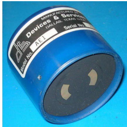
AE1 detector showing the diffuse black heated substrate and the sensing element (center)
