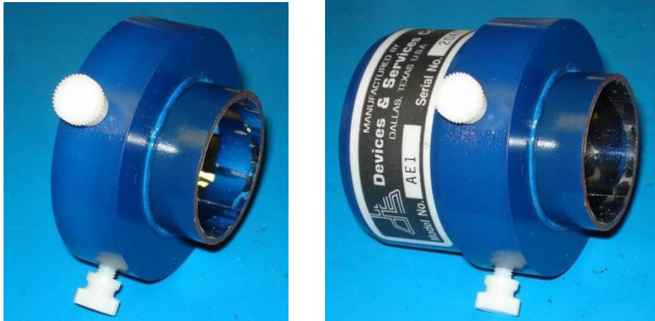
Standard AE-ADP adapter with highly reflective film that redirects radiation heat exchange
