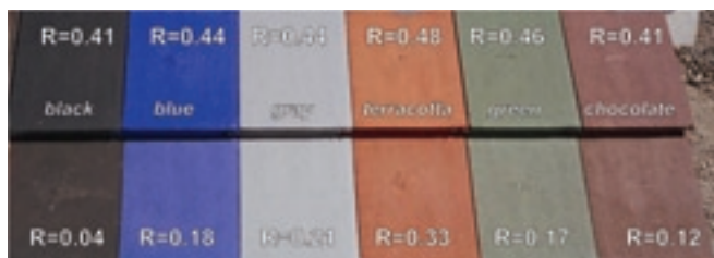
Advancements in pigment technology increase solar reflectance across a broad spectrum. (Photo courtesy of American Rooftile Coatings.)
